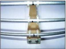
It is a three turn loop closed by a 100PF capacitor covering continuously from 3.5 MHz to 8 MHz
