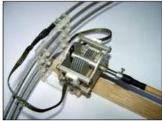
The 40/60/80 is a portable loop that covers 80 meters with a high degree of compromise. I have never opportunity to test on 60 meters.
