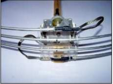
The structure is made on airplane models wood and 5 mms aluminum is used to the loop construction.
