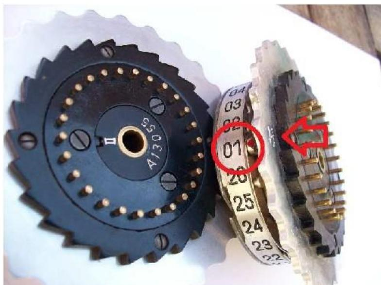
After closing the door, rotate the rotor rings in such a way to read, from the left to the right, the values 09,20,16,or I - T- P (photo 1, Grundstellung).
